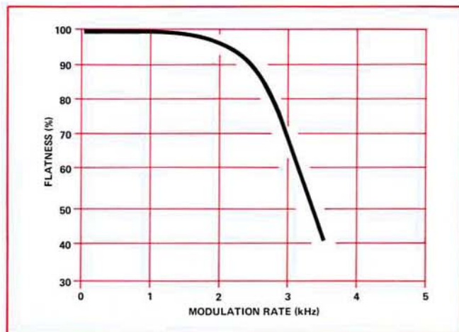
Figure 4-26. Typical 3 kHz low-pass filter response.
